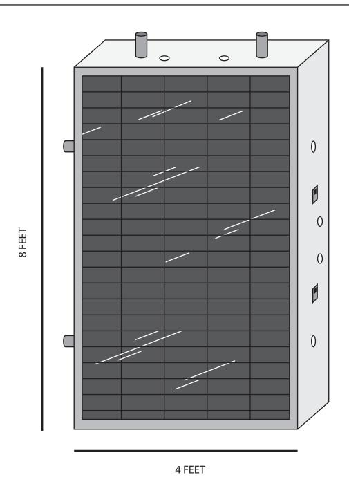
We will begin by producing NOMAD Blocks in standard SIP sizes and dimensions, for cost and efficiency's sake. Additional sizes with be segmented into fractions of the typical 4'x8' SIP, OSB, drywall and plywood cutout dimensions, such as 4'x4' and 2'x2' units. Solar (PV) cells coupled with flashing will double as waterproof siding on the exterior of the panel.
